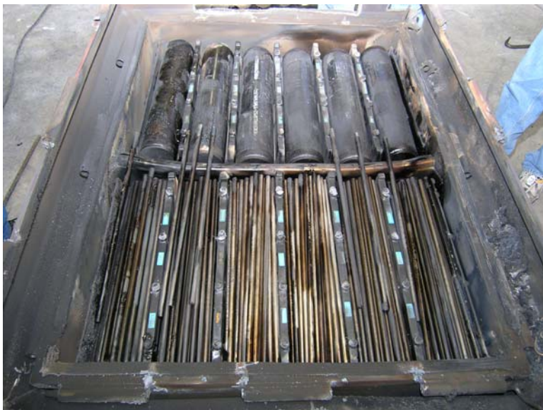
Figure 4 – Payload Condition, Post Drop and Burn Test
