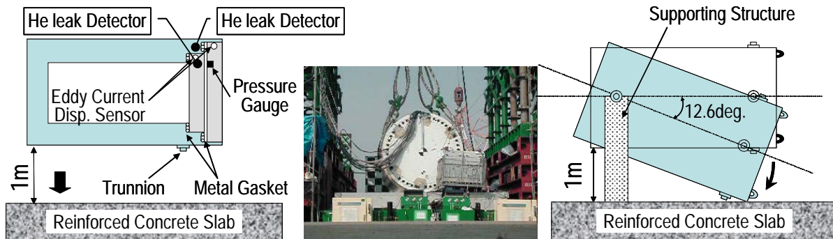
Figure 3. Drop Test Conditions with Full-Scale Metal Cask
