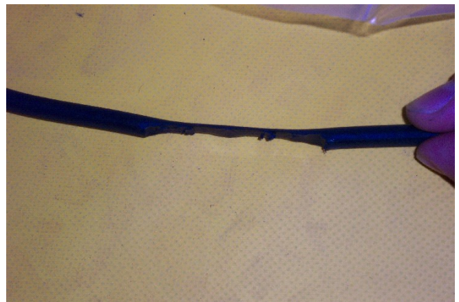
Figure 6: Damaged O-Ring Detail
