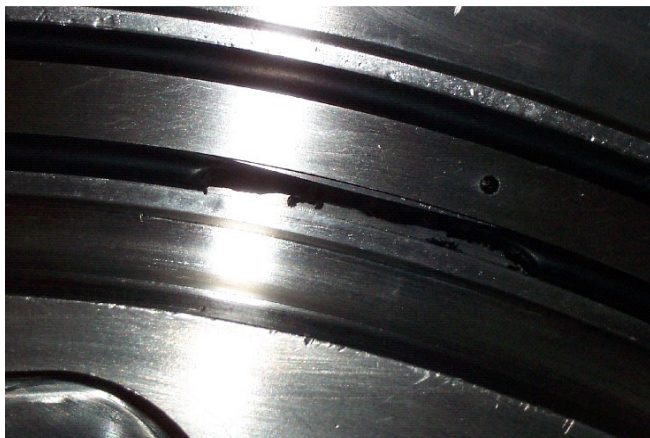
Figure 5: Damaged O-Ring in Groove
