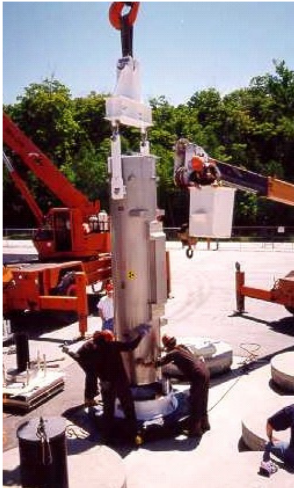
Figure 4: Unloading of the Roadrunner Transportation Package
