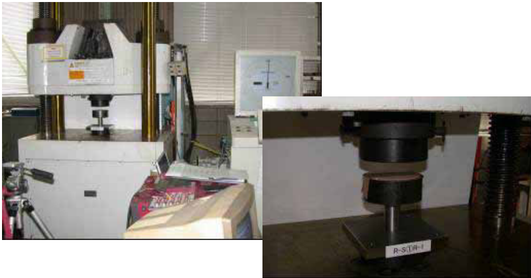
Figure 3. Equipment of static compressive test
