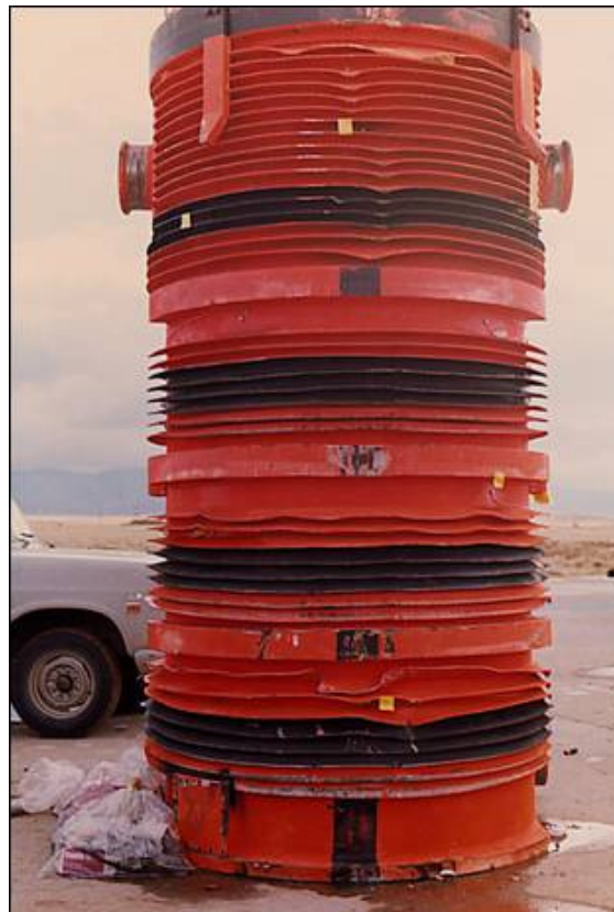
Fig. 1. Photograph of the obsolete 67-tonne cask prior to fire test.
