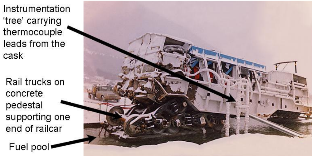
Fig. 5. Cask/railcar assembled over fuel pool prior to testing.
