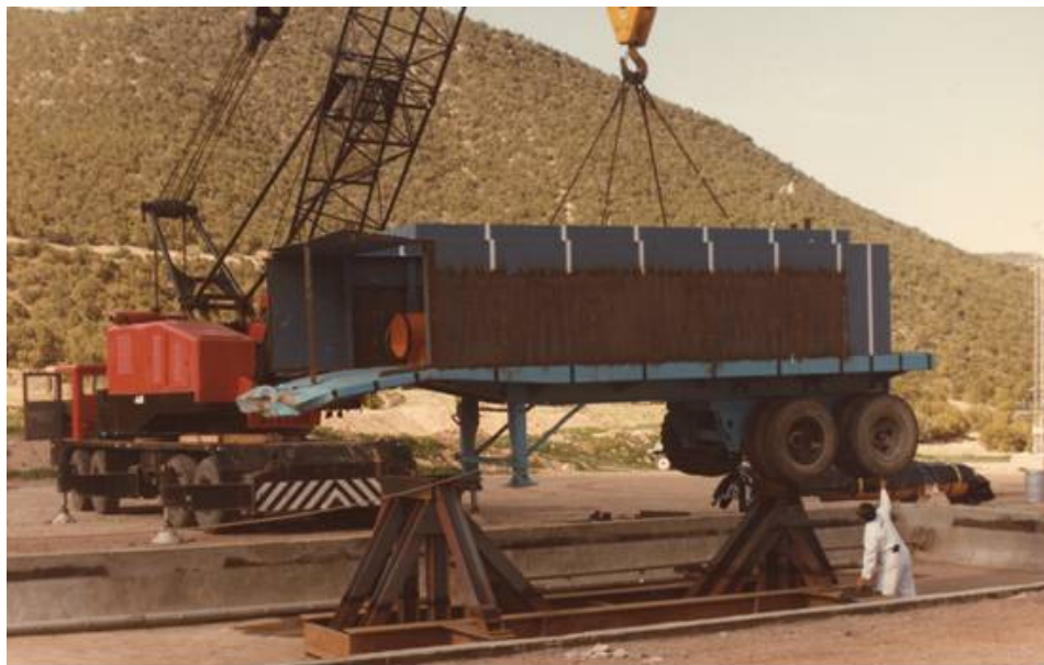
Fig. 6. Placement of SNM cask in tested trailer over fuel pool.
