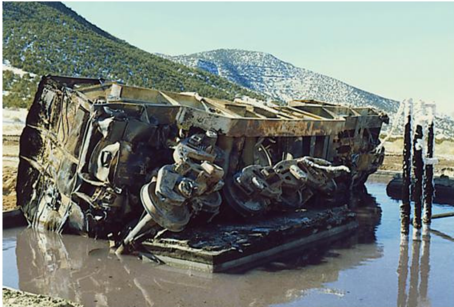
Fig. 8. Cask/Railcar following exposure to fire for 125 minutes.
