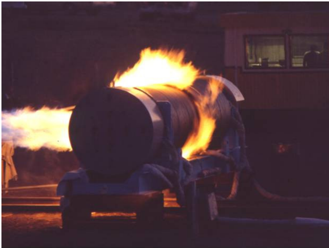
Fig. 11. Photograph of modified HNPF cask being exposed to torch environment at the side of the cask in the centre.
