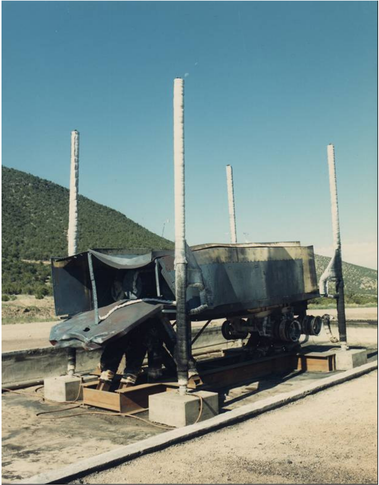
Fig. 10. Photograph of cask/trailer system following fire exposure.
