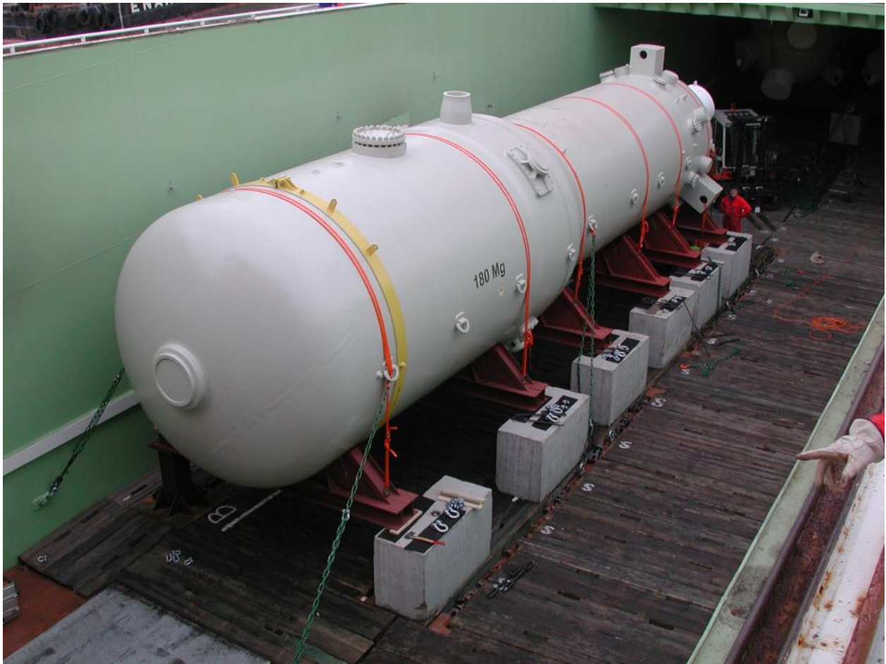
Figure 6. Positioning of the steam generator in the vessel
