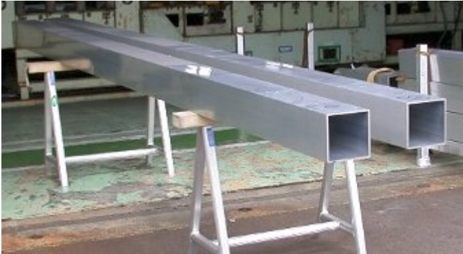
Fig. 10 Sample of square tube in actual size for BWR fuel basket
