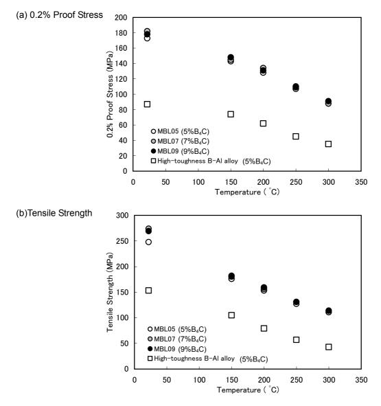
Fig.5 0.2% proof stress and tensile strength of high-strength B-AI alloys
