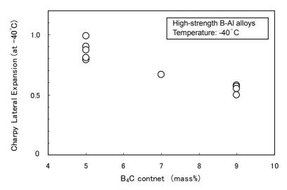
Fig.6 Dependence of Charpy lateral expansion of high-strength B-Al alloy on B<sub>4</sub>C content (tested at -40°C)
