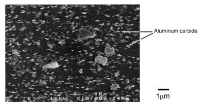
Fig.4 SEM (Scanning Electron Microscopy) micrograph of aluminum carbide particles in MBL09 alloy.
