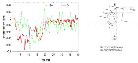
Fig. 6: Sliding (radial) and opening (axial) displacements at the groove of the large metallic seal of the primary lid
