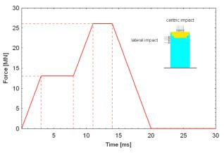
Fig.1: Load vs. time function for the MEPPEN test projectile described in [9]
