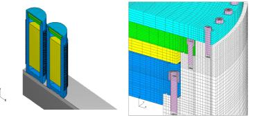
Fig. 7: a) FE-Model with the storage building ground (left) b) Detail of the lid system with its bolts (right)
