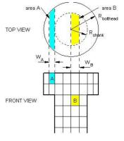
Fig. 2: Cross-sectional views of the bolt head and the shank [11]
