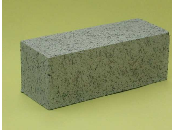
Photo1 Cut sample of heat resistant concrete
