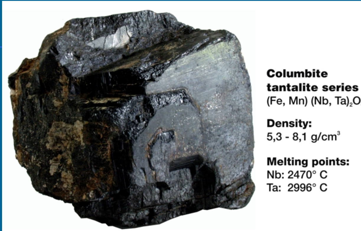
Fig. 2: The mineral Tantalite is the principal source for the production of Tantalum and Tantalum products
