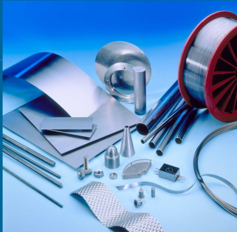
Fig. 9: Components of Tantalum Metal are very resistant to corrosion
