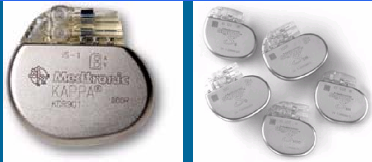
Fig. 4: Heart pacemakers require reliable capacitors, made from Tantalum metal
