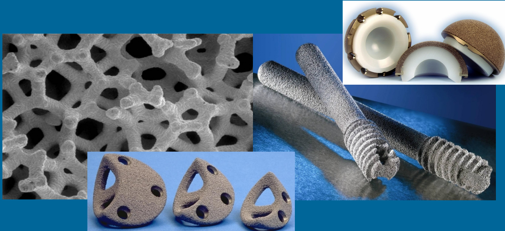
Fig. 8: Tantalum is used for the reconstruction of joints and tissues in the human body, as it is inert to body fluids
