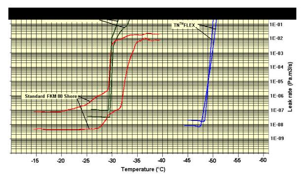
The replication for the two TN<sup>TM</sup>FLEX gaskets tests is very good, <u>the leakage occurs at a temperature below -47°C</u>, which is a significant improvement in comparison with standard FKM grades used by COGEMA LOGISTICS which can guarantee the leaktightness only to -27°C.
