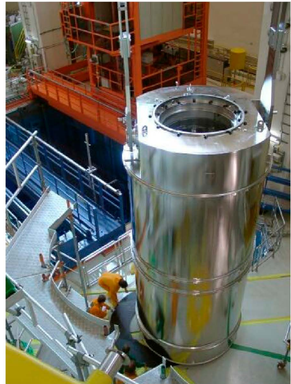
Figure 6 Transport flask fully encapsulated by three part metal skirt
