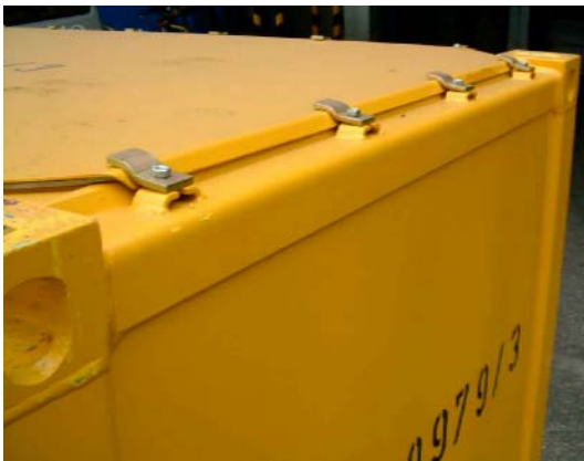
Fig. 5: Lid fixing by T-headed-screws
