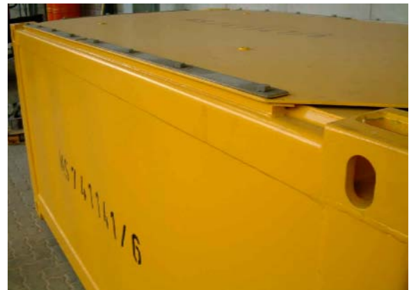
Fig. 6: Improved lid locking system for steel containers
