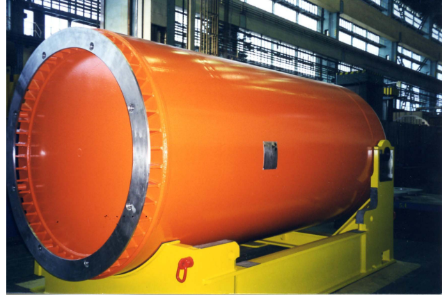
CONSTOR® RBMK a concrete cask for PWR FA
