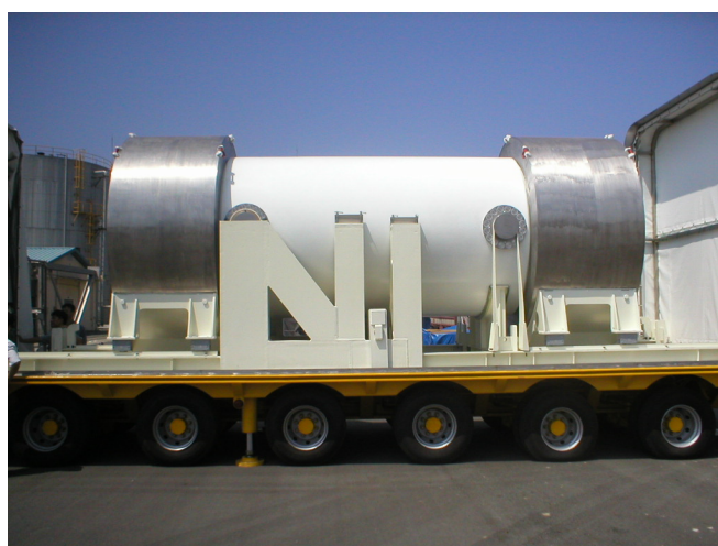
Fig. 3 Cask on the tie-down structure
