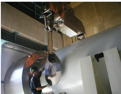
Fig. 6 Cask lifting device
