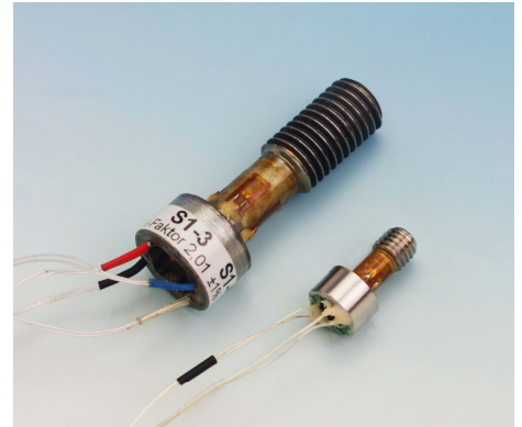
Fig.4: Cask's lid bolts instrumented with strain gauges to determine pre-strain after torquening and loading during impact.
