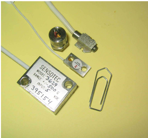
Fig.2: Various miniature, light weight piezoelectric/ piezoresistive accelerometers for high-level mechanical impact measurements.
