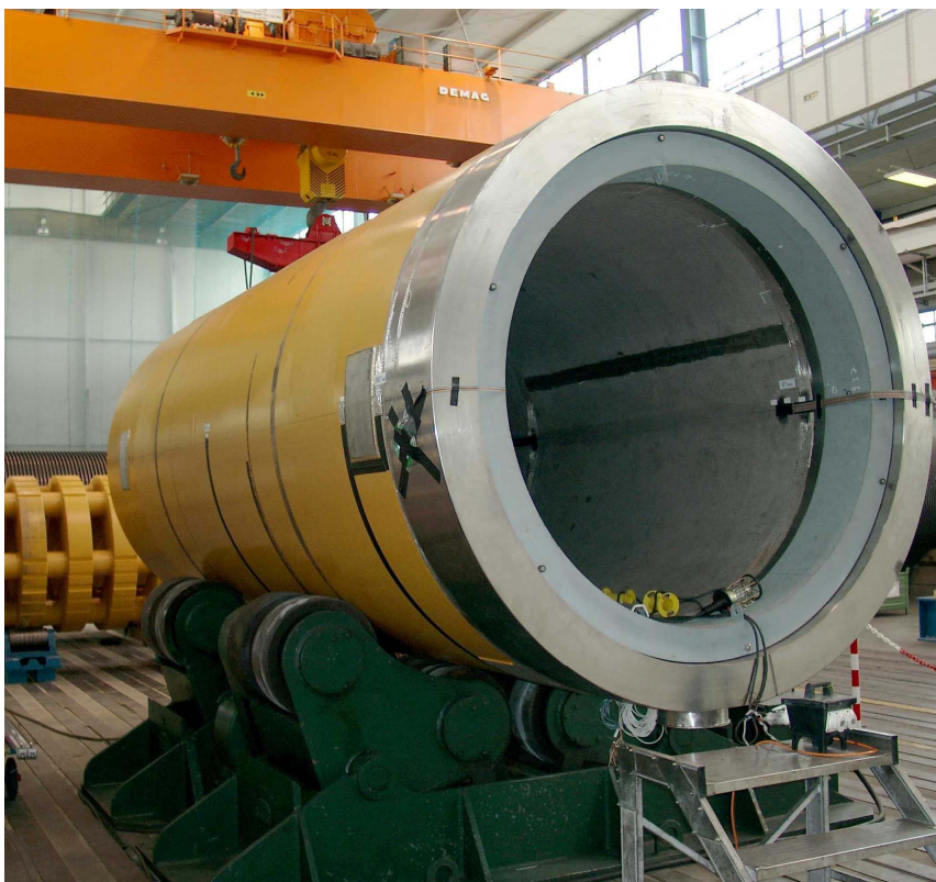
Fig.1: Instrumentation of the cask body with strain gauges and accelerometers
