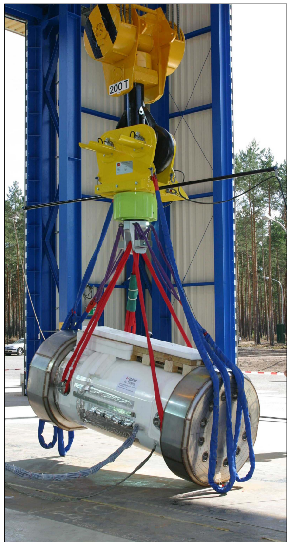
Fig.4: Cask's lid bolts instrumented with strain gauges to determine pre-strain after torquening and loading during impact.
