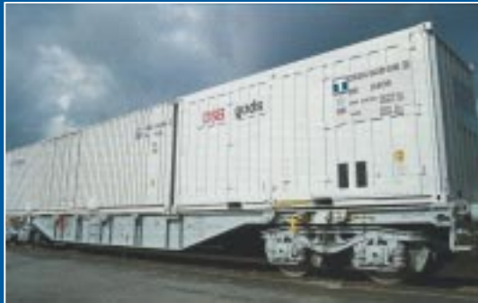
Standard Sgns rail wagon loaded with 20' containers
