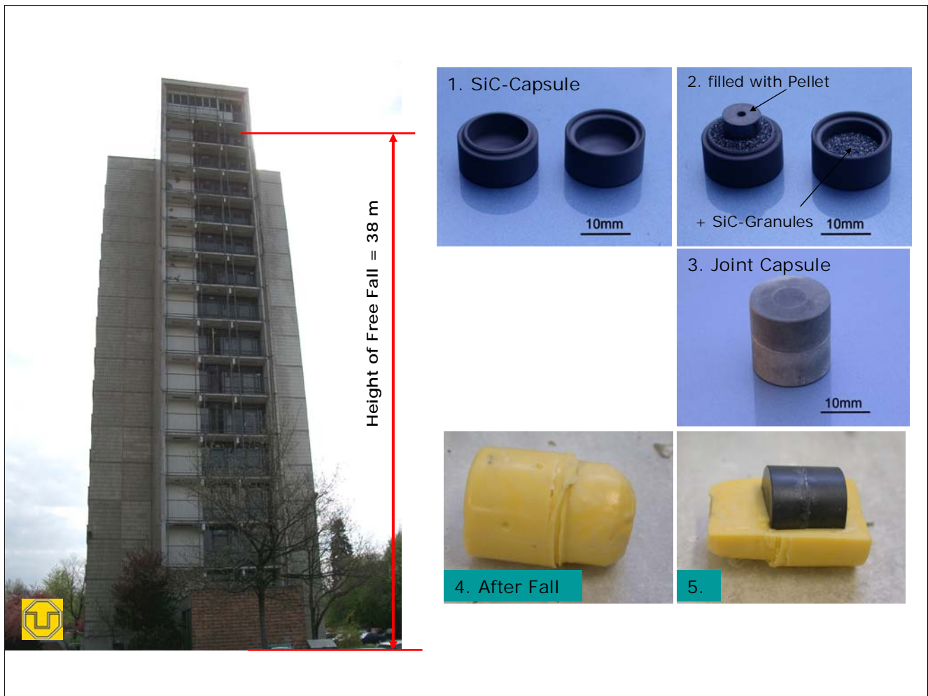
Figure 7 SiC Encapsulated Pellets - Free Fall Tests (Height: 38 m from concrete panel)
