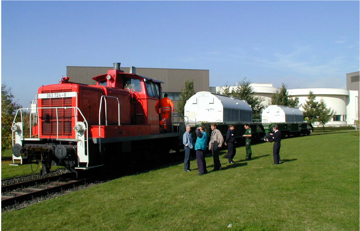
Fig. 2: Two flasks TN 12/2 are ready to leave the KMK Mülheim-Kärlich power station
