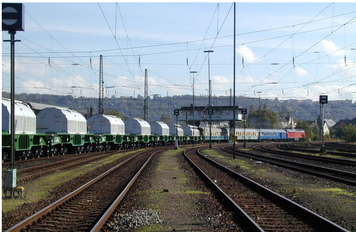
Fig. 4: Dedicated train hauling 7 flasks with spent fuel elements passing station Koblenz-Lützel
