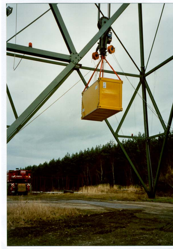
Fig. 4: Type IV package before 5 m horizontal drop test
