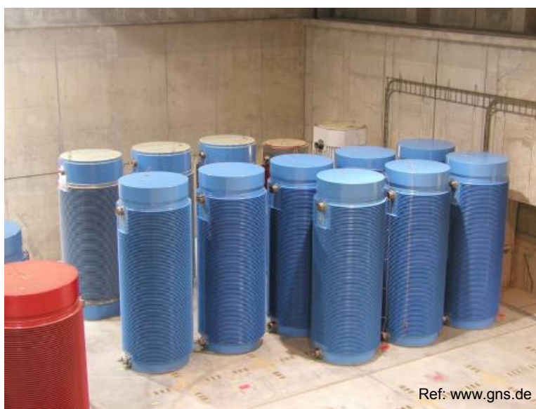
Fig. 1 View on CASTOR® HAW 20/28 CG casks (first two rows) in the Interim Storage Facility at Gorleben
