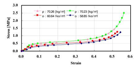
Fig. 4. Compression Stress-Strain Curve of Soft Polyurethane Foam
