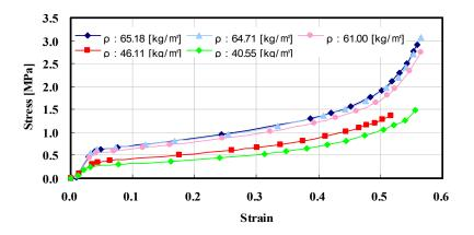
Fig. 5. Compression Stress-Strain Curve of Hard Styrofoam
