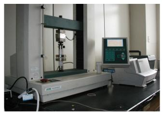
Fig. 1. Compression Tester (Hounsfield, H25K-ST)
