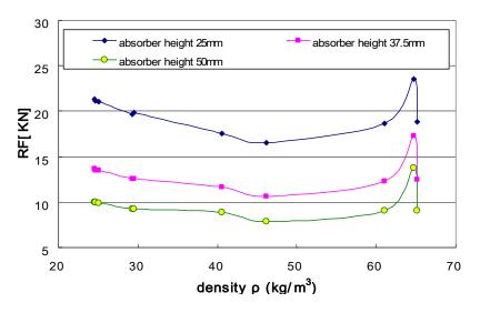
Fig. 8 Reaction Force according to the density
