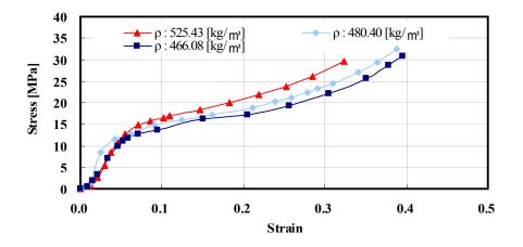
Fig. 3. Compression Stress-Strain Curve of Hard Polyurethane Foam
