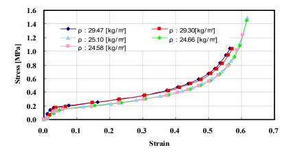
Fig. 6. Compression Stress-Strain Curve of Soft Styrofoam
