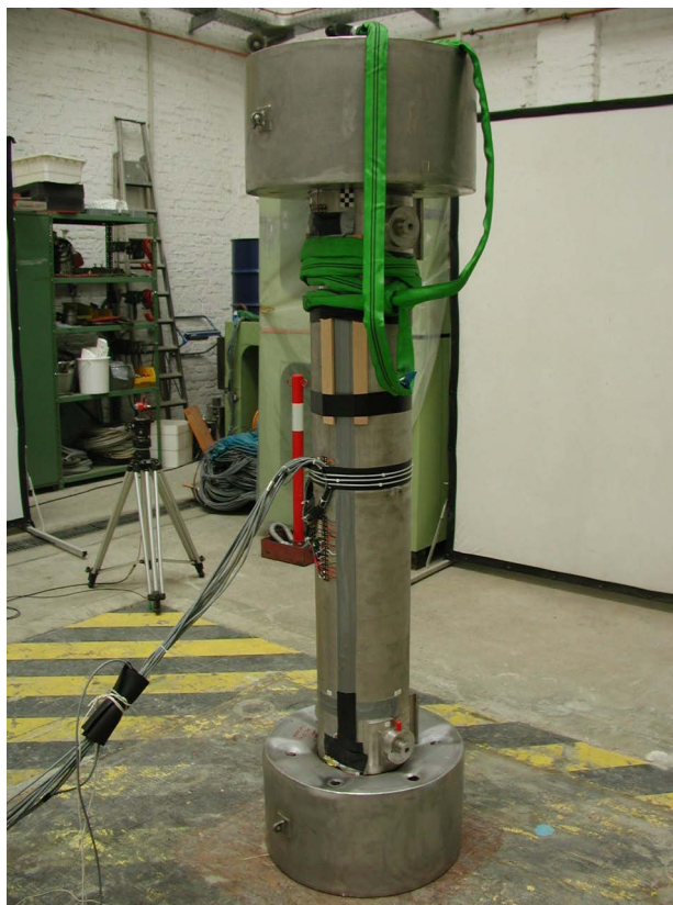
Fig. 2. NCS 45 drop test model after the 0.3 m and 9 m drop test of sequence 1
