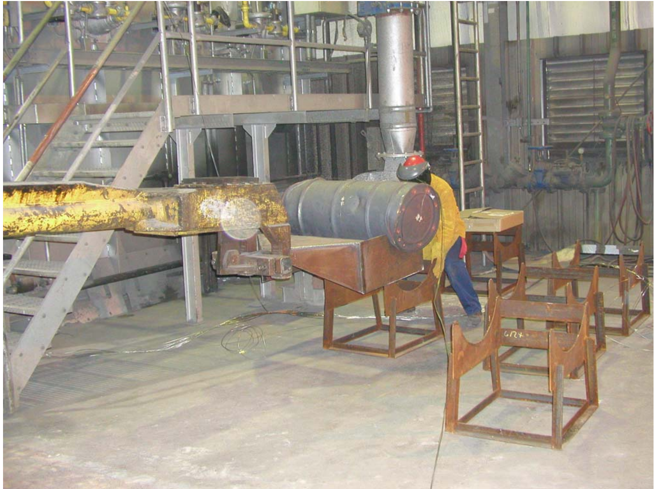
Figure 4. ES-3100 package being placed on a cooling stand at the end of a thermal test
