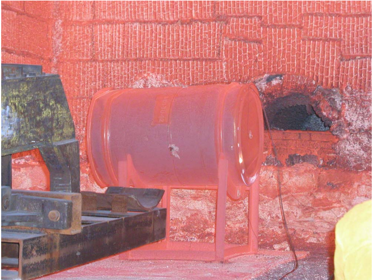
Figure 3. DPP-2 package about to be removed from the furnace at the end of a thermal test
