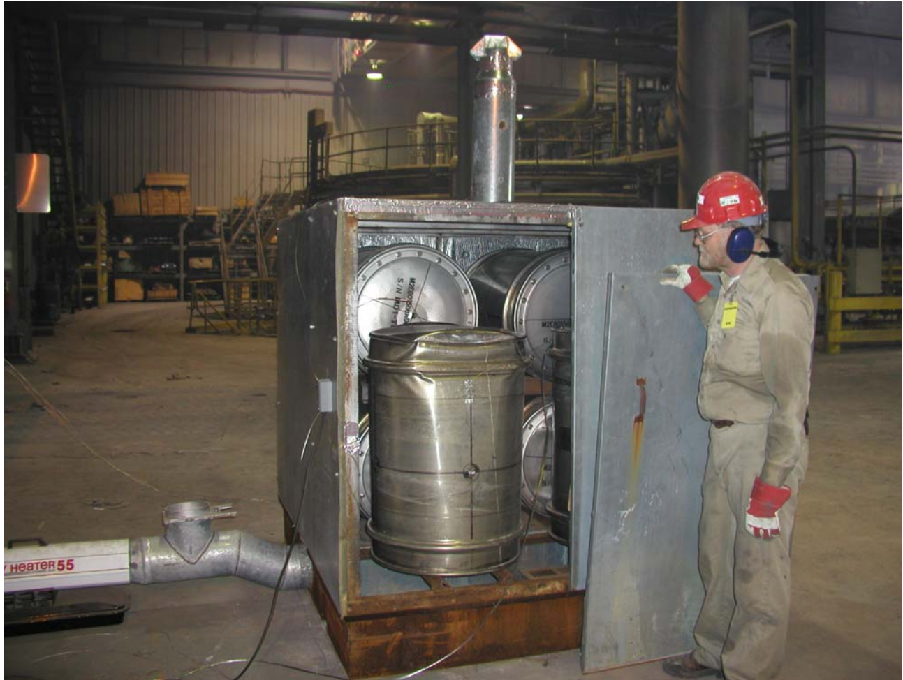
Figure 1. Preheat chamber being used to prepare MD-1 packages for HAC thermal testing
