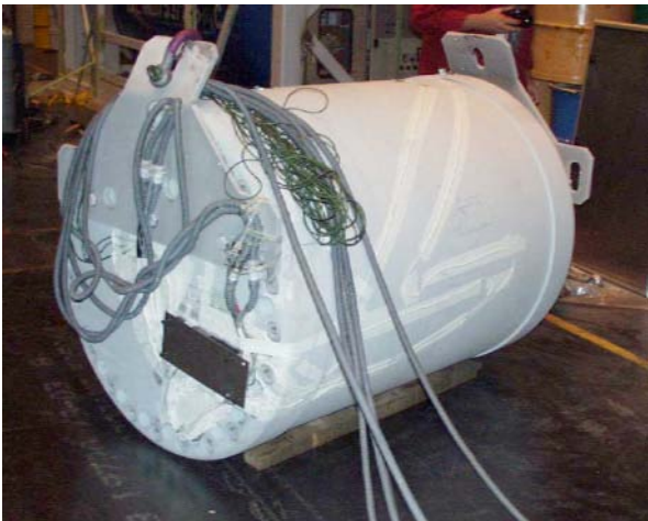
Fig. 4: MOSAIK®II container after drop test
