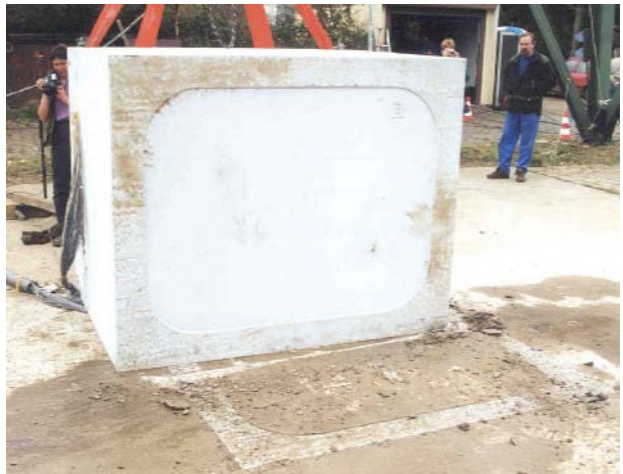
Fig. 5: Cubic container after drop test
