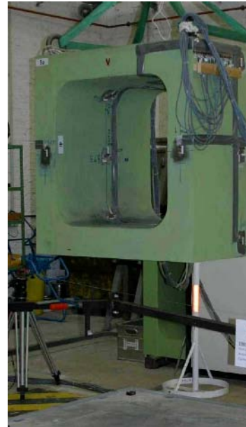
Fig. 7: Drop test of dummy container (Photo courtesy BAM)
