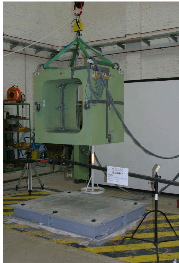
Fig. 1. 1 m drop test with the hollow section A1
