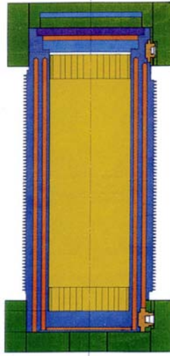
Picture 4: Cask for transport and storage shown with mounted shock absorbers
