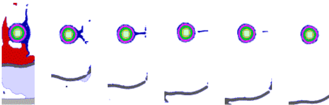
Figure 7. Transverse cross-section views of the deformation of the cask at 2, 5, 10, 15, 20, and 25 ms
