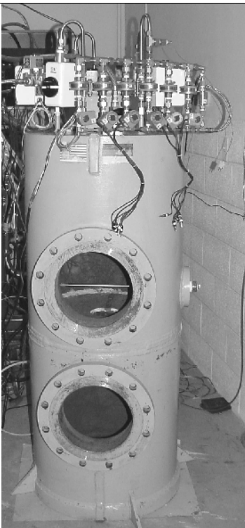
Fig. 1 Phase 2 Test Chamber (open), aerosol chamber (top), with test rod, and explosive containment chamber (bottom)
