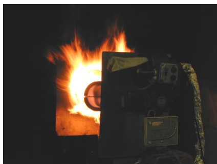
Figure-9 Random packed FR-3718 foam cube test in progress
