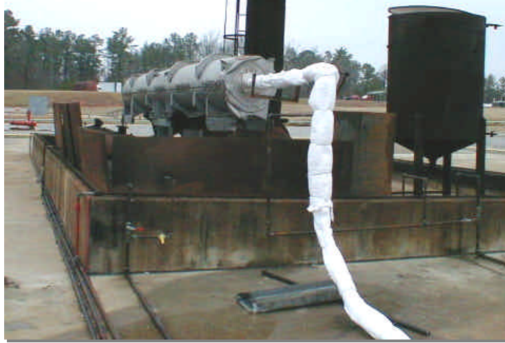
Figure 1 Test Article Before Burn Showing Insulation Wrapped Thermocouple Leads
