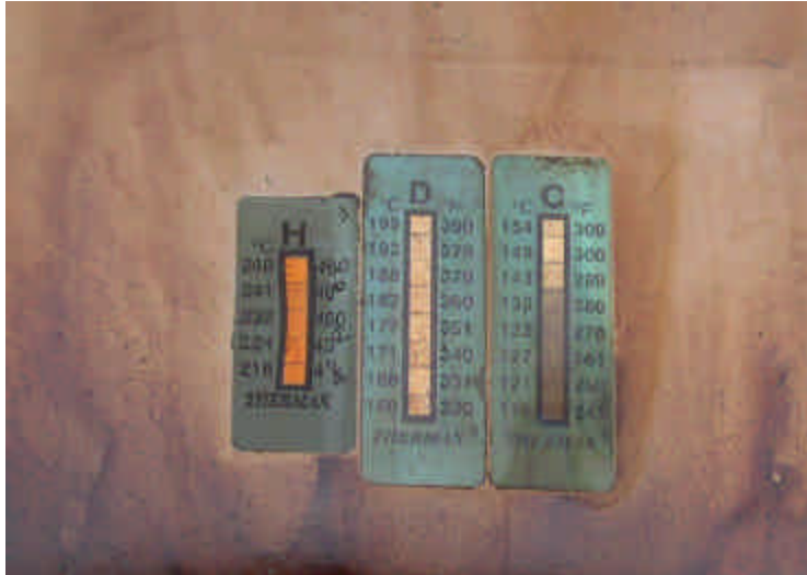
Figure 11 Temperature Strips Inside the Package
