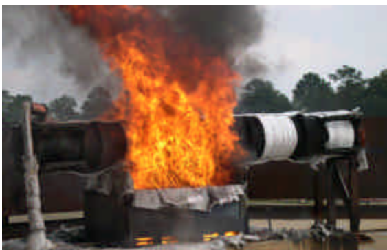
Figure 8 Partial Package Burn Tests
