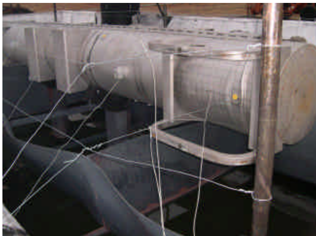
Figure 10 Thermocouples Connected to Outerpack
