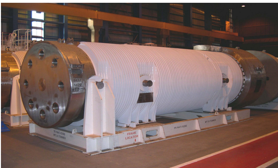
Fig 3 Excellox 4 Flask in Storage at Sellafield
