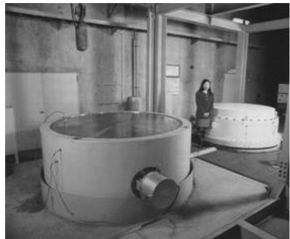
Fig. 3.4.1 Long-term containment tests using full-scale lids of metal cask
