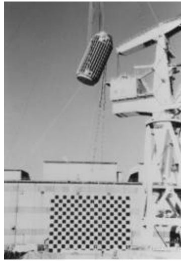
(b) Tilted drop test from 17 m high
