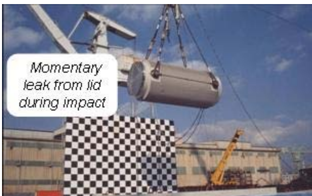
Fig. 3.6.1 Concept of drop test of metal cask without impact limiters
