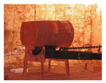
Figure 4. Thermal (Furnace) Test of the Type B Package
