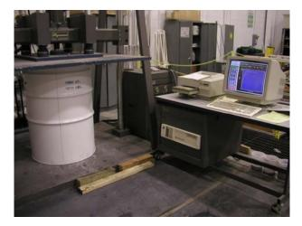
Figure 5. Compression Test of the BRM Shielded Over Pack
