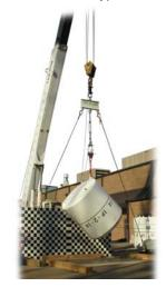
Figure 6. Corner Drop of the Fernald Silo IP-2 Waste Package at NTRC
