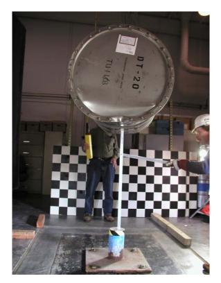
Figure 3. Puncture Test Preparation of the DT-20 Inside the PRF
