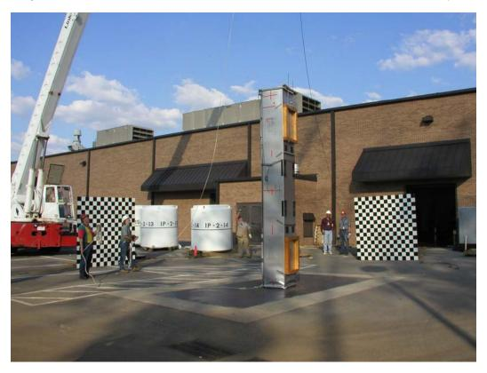
Figure 7. 9-m Drop Test of the RAJ-II BWR Fresh Fuel Package (Perfect Drop)
