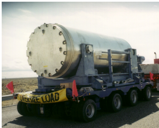
Figure 8: NUHOMS® OS197 Transfer Cask en Route to ISFSI
