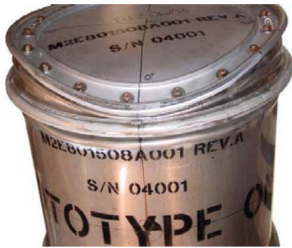
Figure 4. Top view of DPP-2 Test Unit 2 after CG-over-corner tests
