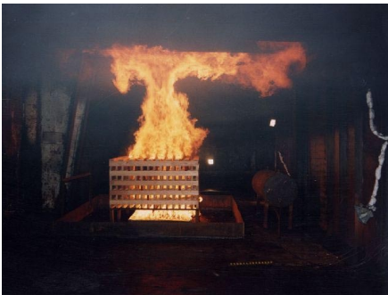
Fig.7 Wood crib fire test in the vessel hold
