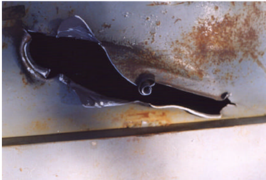
Damage to NAC IP-2 "Strong tight" Package
