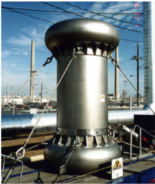
Figure 3. Model GE-2000 for Spent Fuel Shipment.
