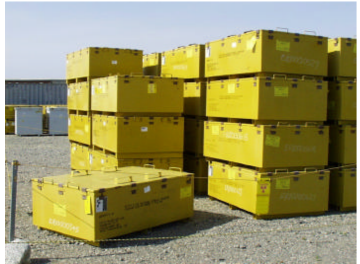
Figure 4. Industrial Packages for LLW and MLLW.
