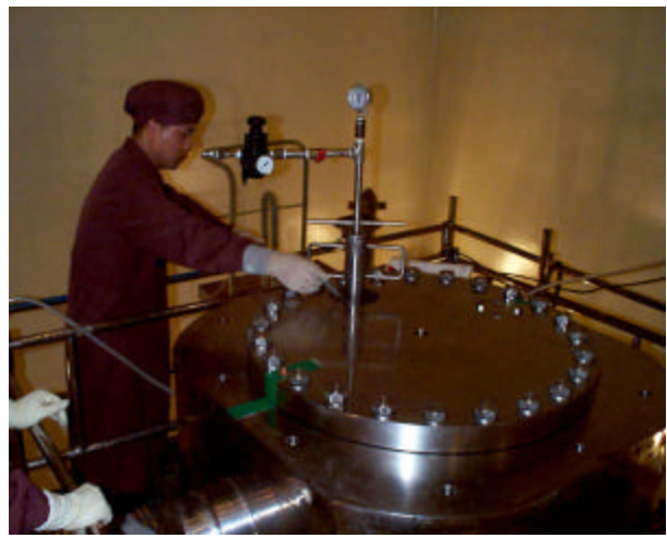
Figure 4 Helium leak test
