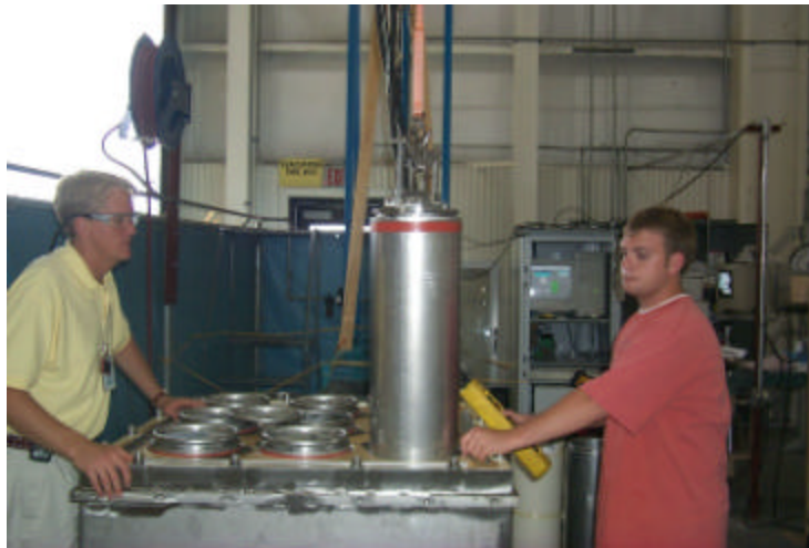
Figure 8b. ICCA removal using overhead crane
