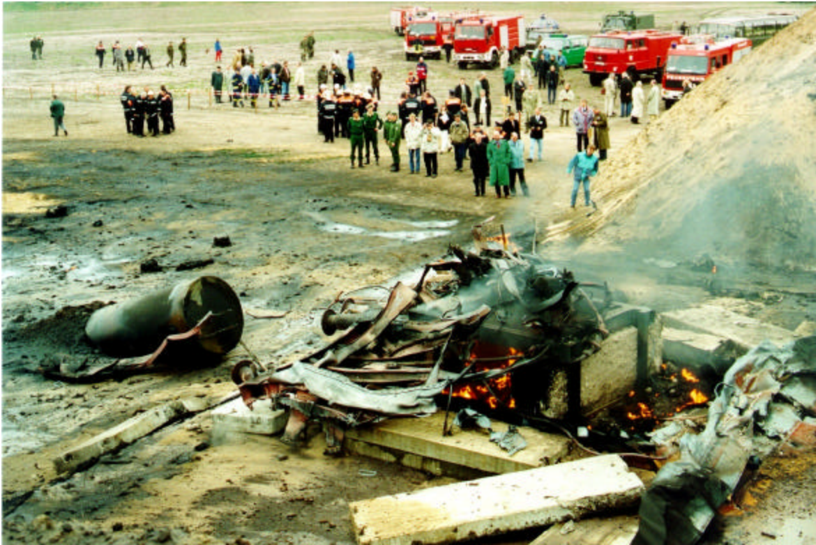
Figure 4. Fragments of the Rail Tank Carriage after the LPG Tank Explosion
