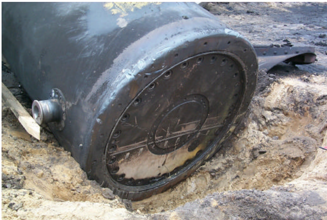
Figure 3. Excavated Lid Side of the CASTOR Cask with Imprints of the LPG Tank Support Saddle on the Outer Lid of the Cask
