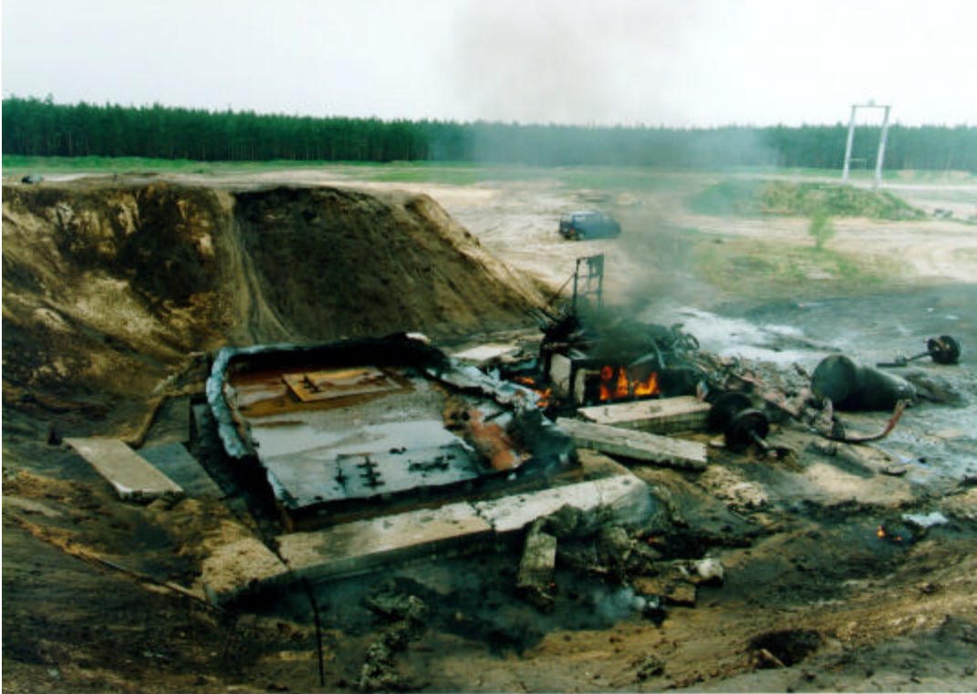
Figure 2. View of the Test Facility a) Before the Test (above): Propane Tank (left) and CASTOR Cask (right) above Fuel Oil Pools b) After the Propane Rail Tank Explosion (below)
