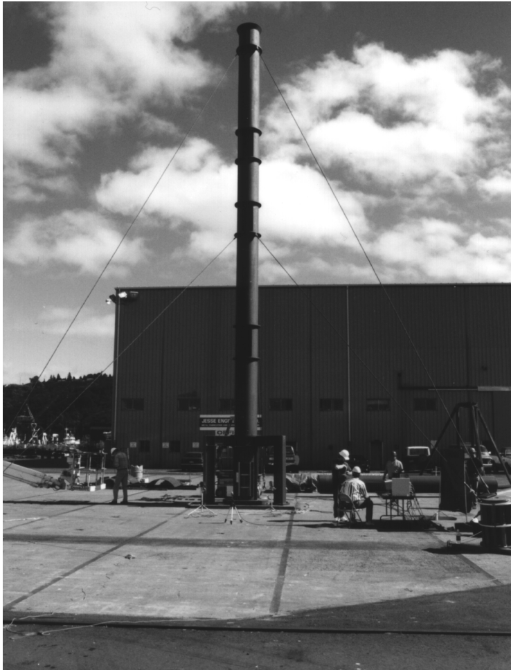
Figure 3 Impact Absorber Prototype Test Setup
