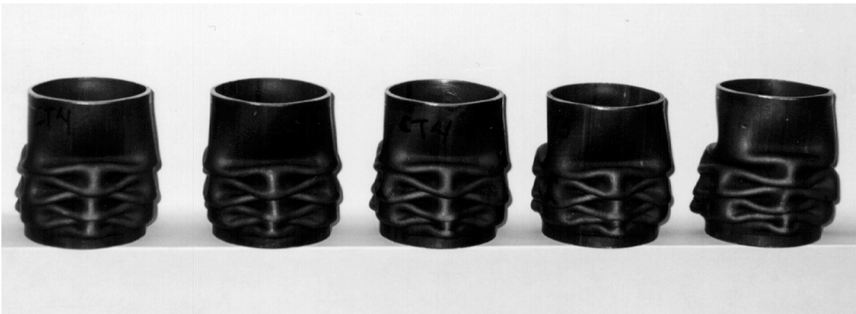
Figure 2c Three-Lobed Deformation Mode
