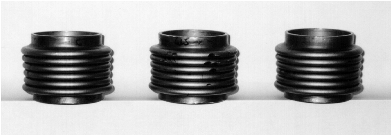
Figure 2a Concertina Deformation Mode
