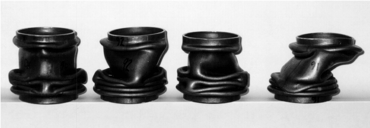
Figure 2b Two-Lobed Deformation Mode
