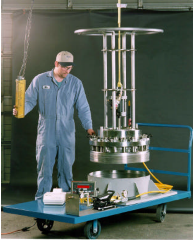
Fig. 2 MCO Closure Tool
