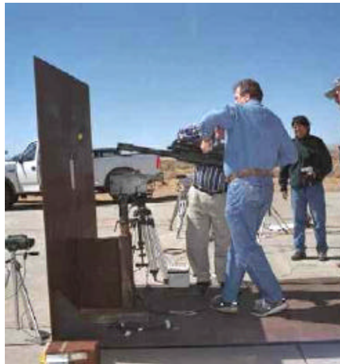
Figure 5, Test Set-Up for Model Mark 19 Grenade Launcher
