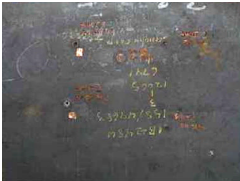
Figure 8, First Plate Penetrated with Armor Piercing Munition
