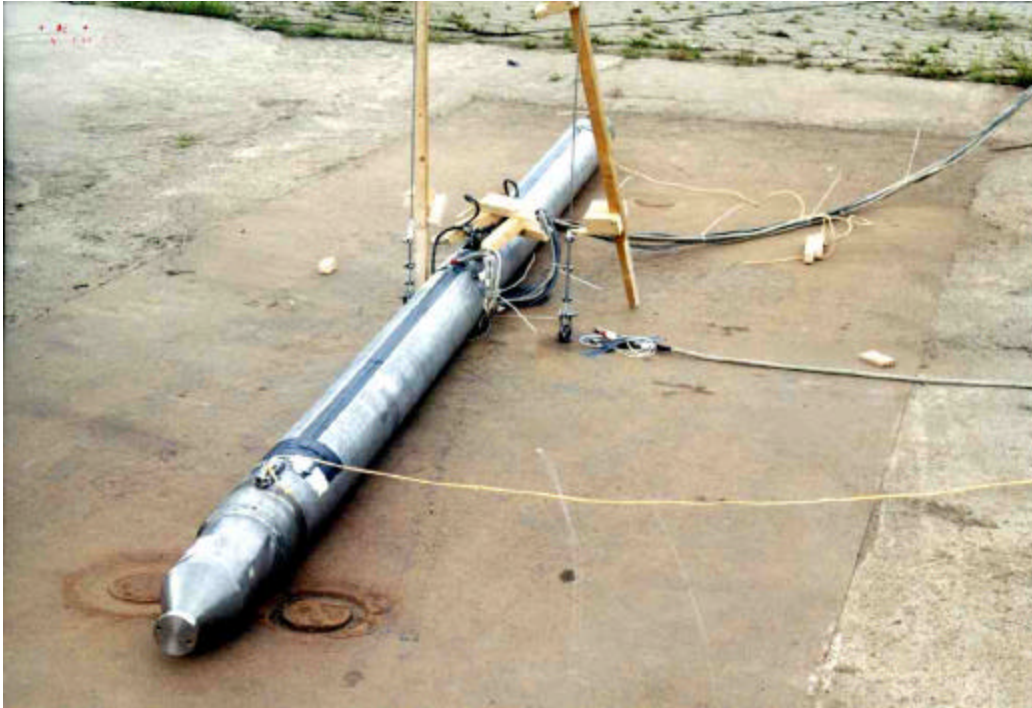
Figure 3: Prototype 3 after the 9 m vertical drop test
