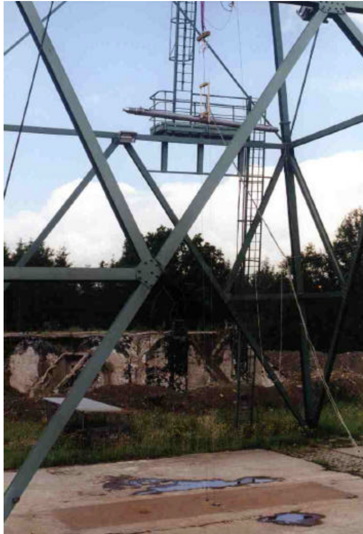
Figure 2: Prototype 3 before the 9 m vertical drop test
