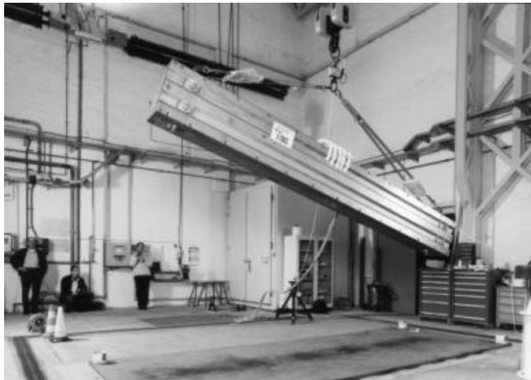
Fig. 4 ANF-10 Drop Test from a Height of 1.3 m
