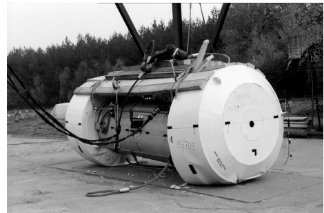
Fig.10. A CASTOR VHLW cask after the 15° declined, 9 m drop test onto a rigid target. In the foreground the higher damaged shock absorber caused by slap-down impact.
