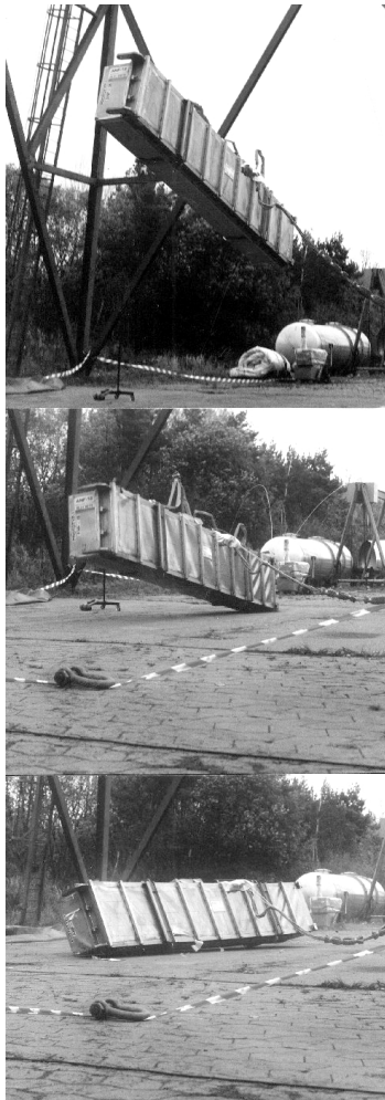
Fig.11. ANF-18. 9 m and 15° declined drop test.
