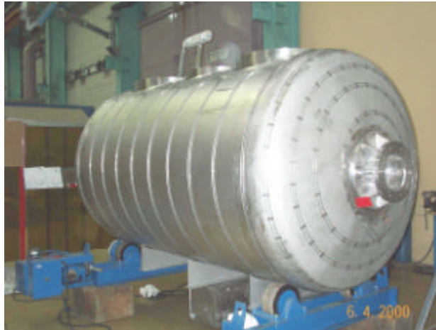
Fig. 3. Internal shell with electrical resistance
